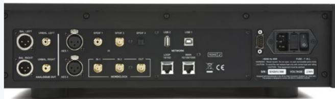
△ NO STONE LEFT UNTURNED IN TERMS OF CONNECTIVITY. MULTIPLE DIGITAL INPUTS CATERING TO ALL TYPES OF DELIVERY, NETWORK PROVISION, WORD CLOCK IN/OUT AND ANALOGUE OUTPUTS (BOTH XLR AND RCA) FOR DIRECT HOOK-UP TO AN INTEGRATED OR POWER AMPLIFIER.
